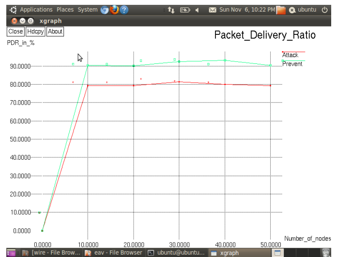
Figure 7. Comparing the packet delivery ratio for eavesdropping attack in at attack time and after prevention attack
