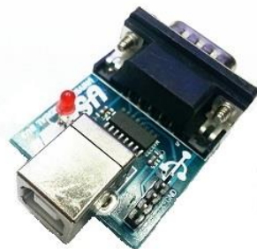
Fig. 7 USB TO SERIAL/UART
