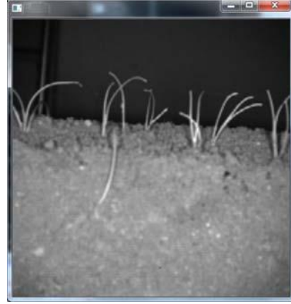
Fig. 3. Original image of the ToF camera with a resolution of 204 \times 204 pixel.
