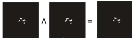
Fig 5. The image after applying the logical AND operation on the RE image and the tophat image
