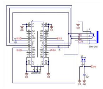
and CC2 pins. These resistors on the CC lines are directed by the USB Sort C determination. The four simple sound signs are a similar which are being utilized by a customary 3.5 mm headset jack. This connector makes it conceivable to interface existing simple headsets with a 3.5 mm to Sort C connector for this show. The connector likewise gives a couple of 1k ohm (Ra) pull down resistors. The accompanying chart demonstrates the case schematics of an aloof 3.5 mm jack to the Sort C connector.
