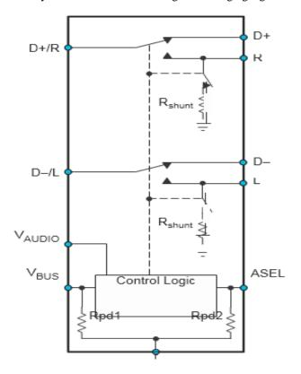
The TS3A227E is used particularly to automatically detect and orient the MIC and GND signals of the 3.5 mm jack to support the function described in the USB Type-C standard above. The USB Type-C to 3.5 mm dongle is on the sink side of the system, therefore, the system user may connect speakers or a headphone set to listen to the audio. Headphones often come with a 4-pole
