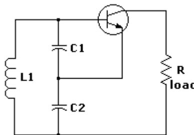
Figure 2 - schematic of a collpitts oscillator
